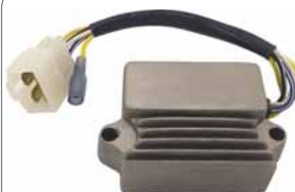
JRG402 KB-4S Boxer- CT / CT-100 4 Pin Socket + 1 Terminal
